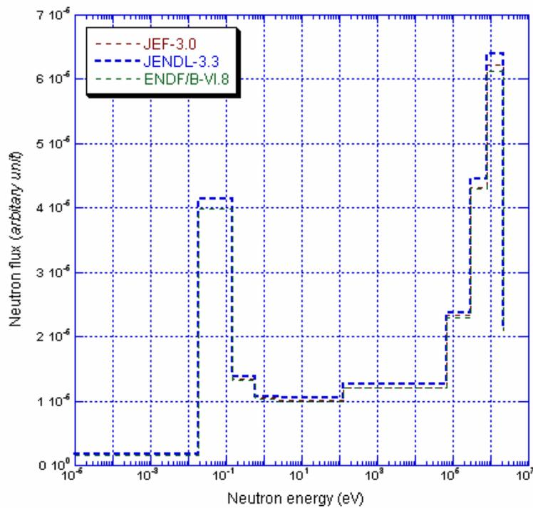
FIG. 6. Neutron flux distribution at a selected standard fuel element
