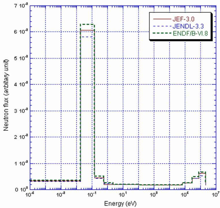
FIG. 5. Neutron flux distribution at a selected beryllium reflector element
