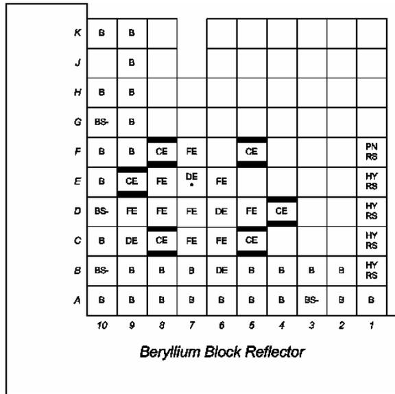
Note : FE = Fuel Element, CE = Control Element, B = Be Reflector Element,
