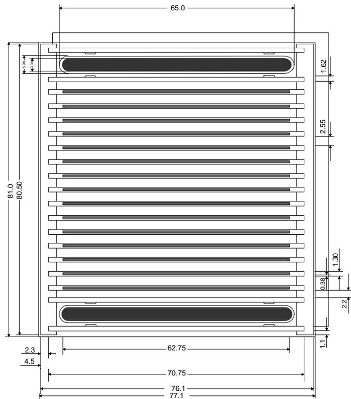
FIG. 2. RSG GAS control fuel element (unit mm)
