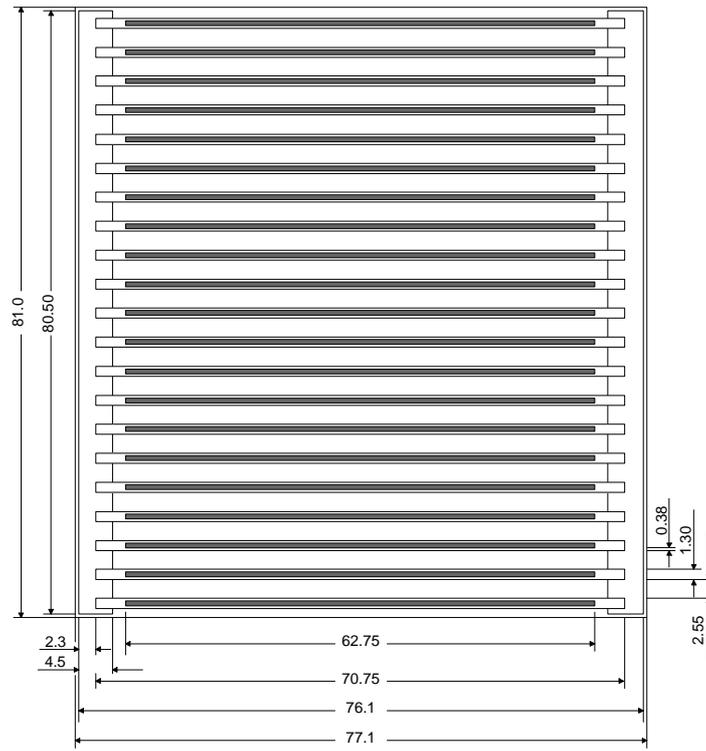
FIG. 1. RSG GAS standard fuel element (unit mm)
